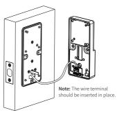
7、Fix the rear panel with three M4x16 screws. Make sure the twist is vertical.
